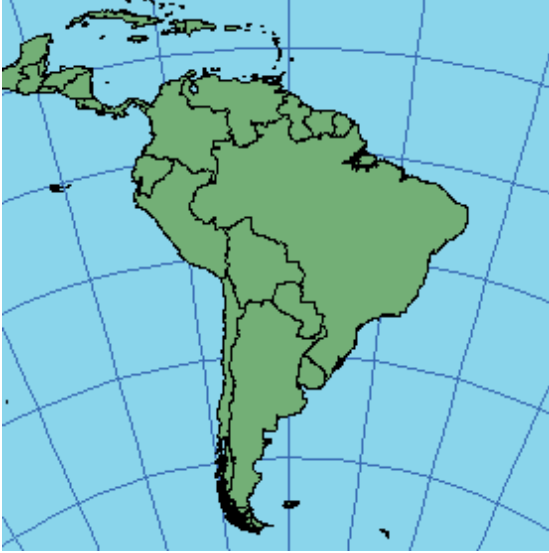
The central meridian is 60° W. The first and second standard parallels are 5° S and 42° S. The latitude of origin is 32° S.
