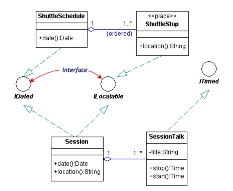
In circle notation, the interfaces are circles with lines connected to the implementing classes. Since it is more compact but leaves out some detail, the lollipop notation simplifies the original diagram.
