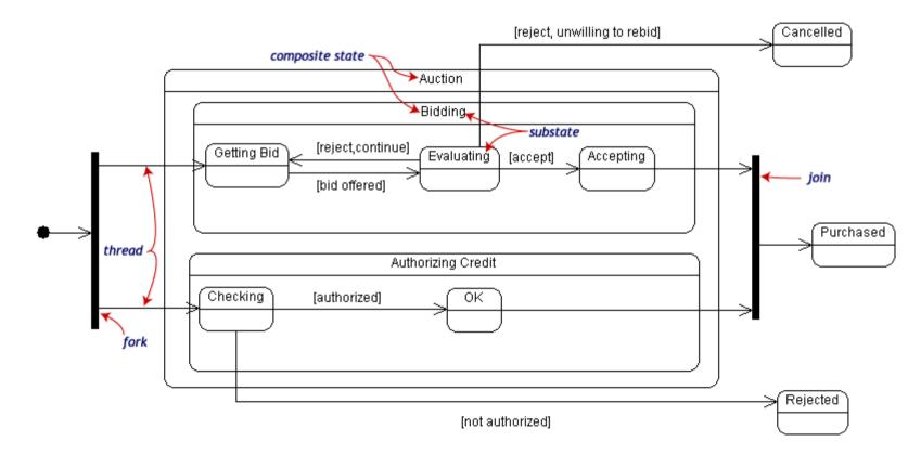
Entering the Auction requires a fork at the start into two separate threads. Unless there is an abnormal exit (Cancelled or Rejected), the exit from the Auction composite state occurs when both substates have exited.
