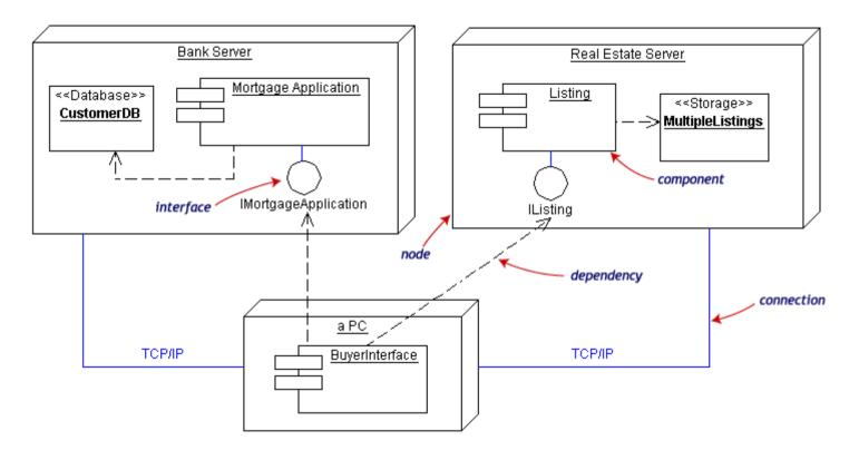
The physical hardware is made up of **nodes**. Each component belongs on a node. Components are shown as rectangles with two tabs at the upper left.
