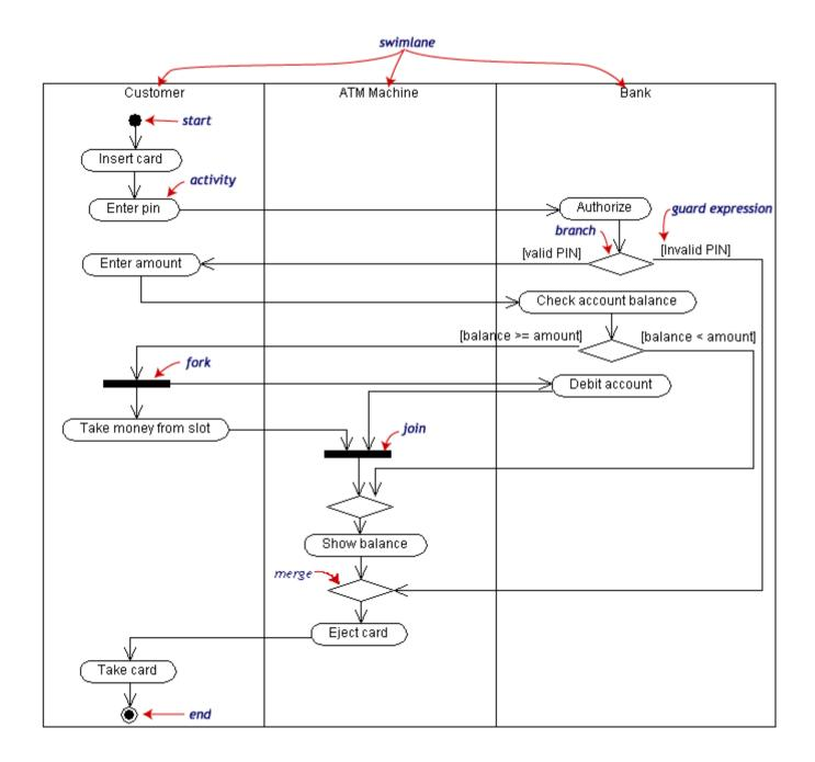
Activity diagrams can be divided into object **swimlanes** that determine which object is responsible for which activity. A single **transition** comes out of each activity, connecting it to the next activity.
